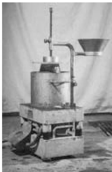
Figure 19.7 The Vebe Test
