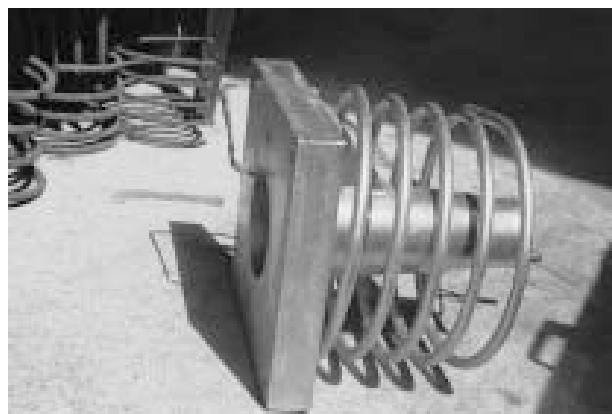
Figure 17.4 Typical beam anchorage
