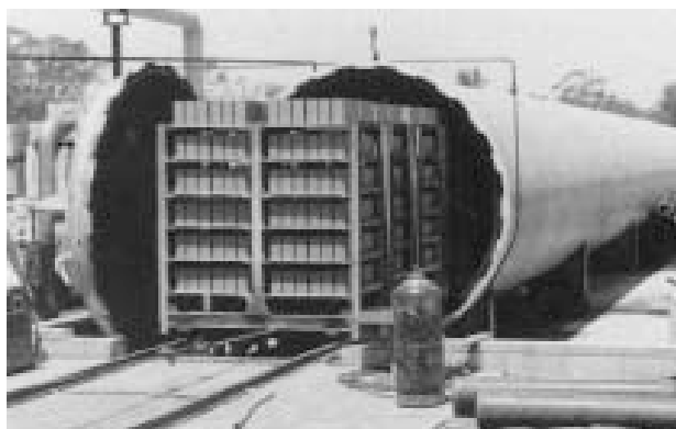
Figure 11.11 Autoclaving concrete blocks
