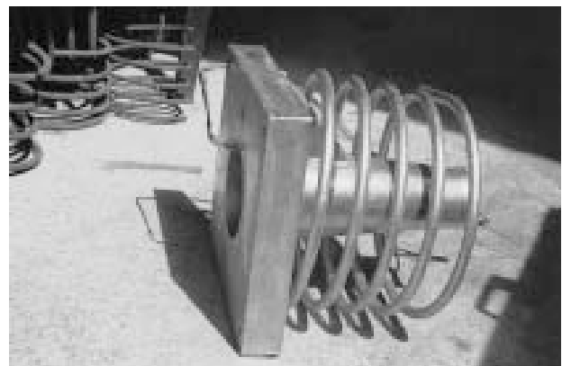
Figure 1.19 Typical beam anchorage
