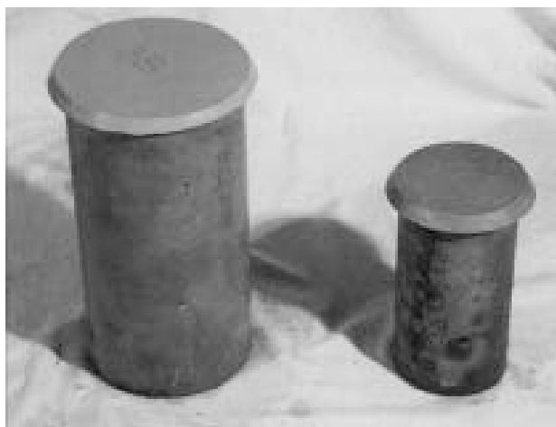
Figure 21.9 Capped concrete test cylinders in each of the two sizes
