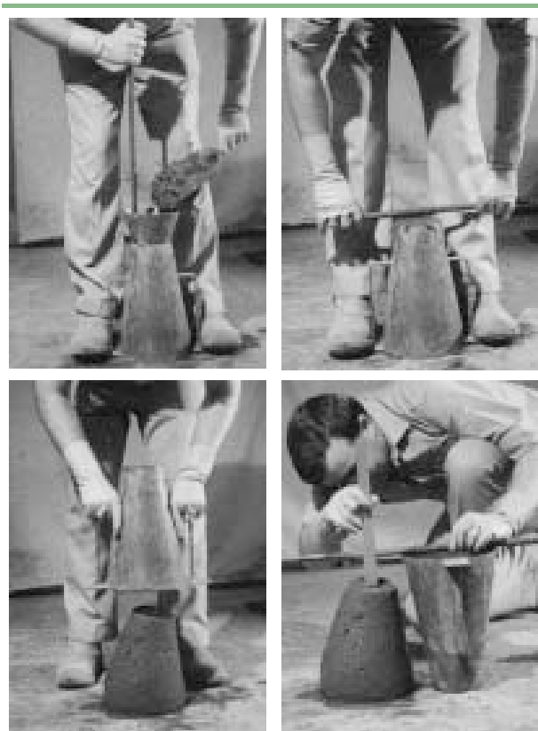
Figure 19.4 The slump test
