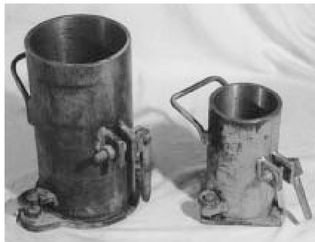
Figure 21.8 Moulds for the two sizes of concrete test cylinders
